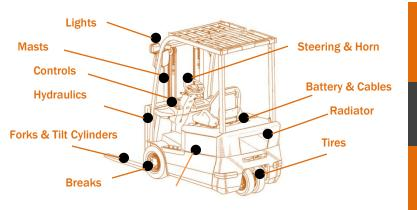
Forklift drivers must inspect the forklift daily prior to start of the shift.
